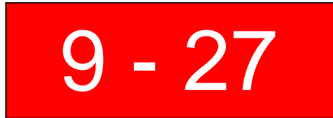
Runway Hold Sign
