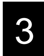
Runway Distance Remaining Signs
